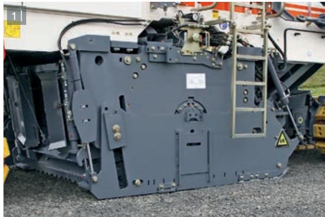
1 | In lowered position, the side plates move over the surface.
