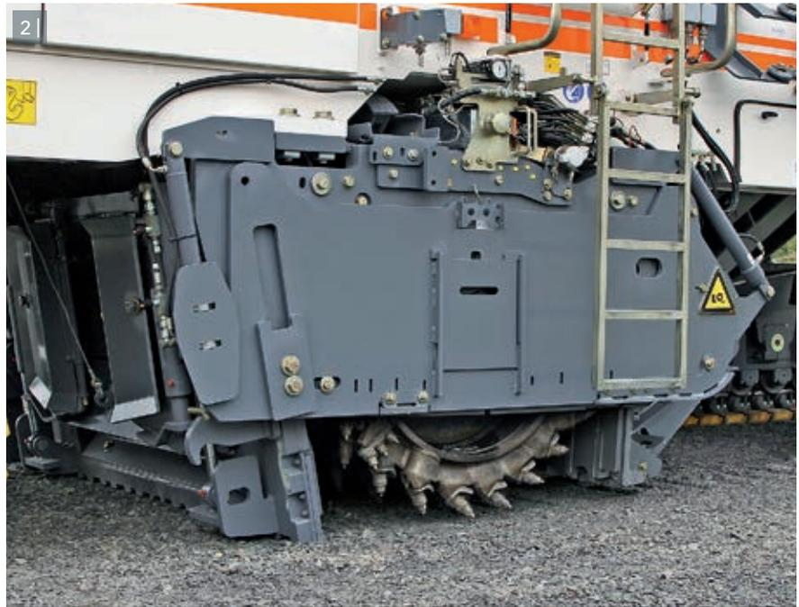
2 | In raised position, the side plates enable the road surface to be milled off accurately along kerbs.
