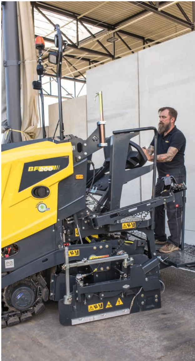
Low position: perfect for extremely confined spaces.
