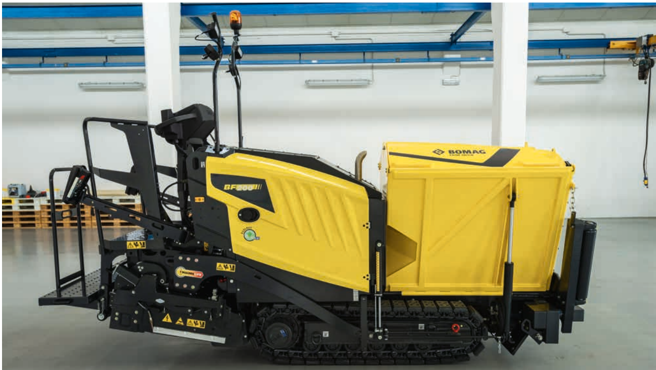
Individually controllable chains allow turning in the tightest of spaces.
