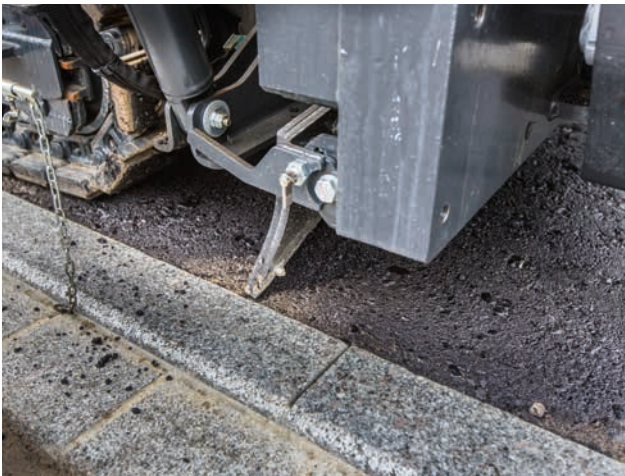
Chain scrapers guarantee low maintenance.
