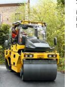
Applications: The tyres of the combination rollers have an intensive kneading effect on the asphalt producing homogeneous compaction and a good surface
