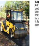
All Typeeical asphalt layers in road construction and service road construction, as well as for use on car parks and access roads, for anti-frost material and light earthworks. The new series -50 is particularly well designed and easy to operate. It features a generous sized operator's platform, either with a comfortable, spacious cab or ROPS.
