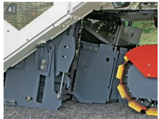
4 | Swing-open baffle plates conduct the recycled material between the rear track units.
