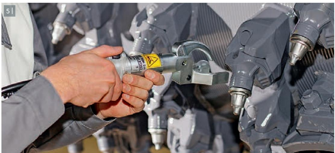
5 | The effective hydraulic cutting tool extractor ensures extremely easy handling with only little effort required.
