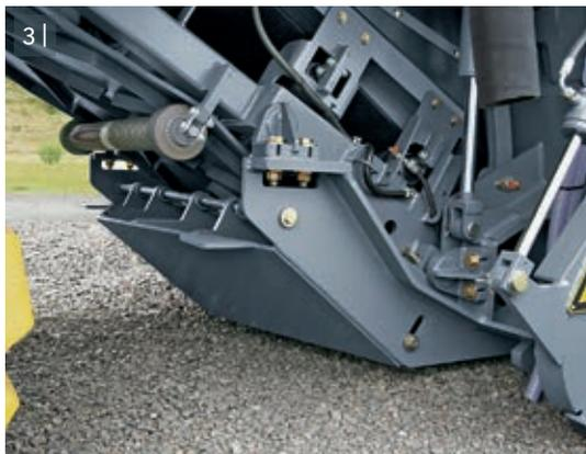
3 | The heavy-duty gradation control beam protects the conveyor belt and prevents the material from breaking into larger slabs.
