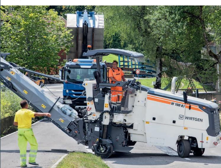
When pivoted in front of the milling drum, the right-hand rear wheel allows precise milling along obstacles such as kerbs or walls.
