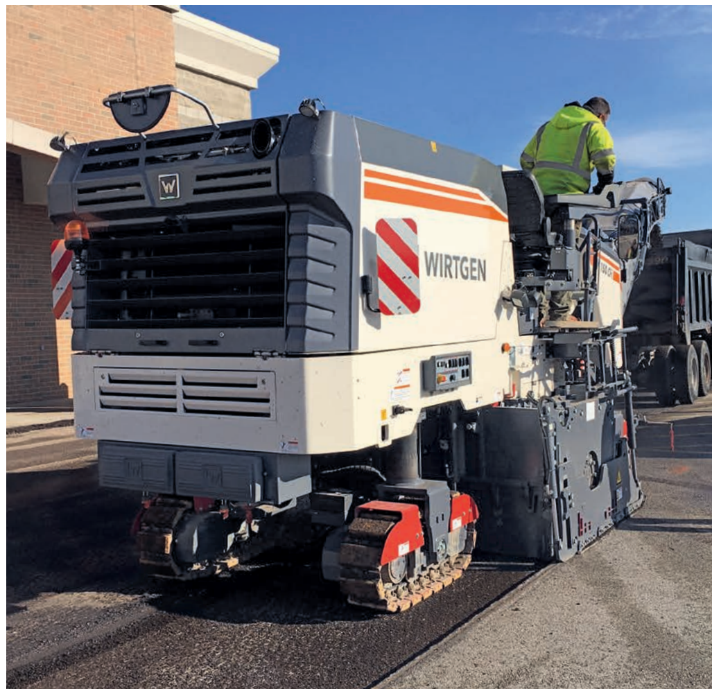
Milling drum Milling width: 1,800 mm Milling depth: 0-330 mm Pick spacing: 18 mm
