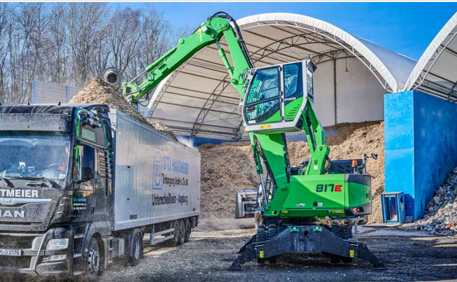
817E - ideal for indoor use/truck loading with compact dimensions and elevating cab
