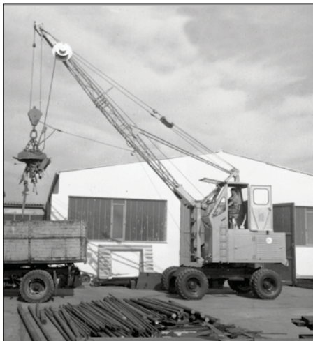
1962: rope-driven S833 with elevated operator cab
