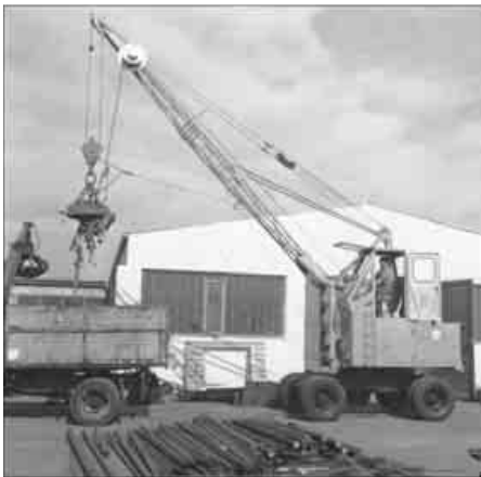
1962: Rope-driven S833 with elevated operator cab
