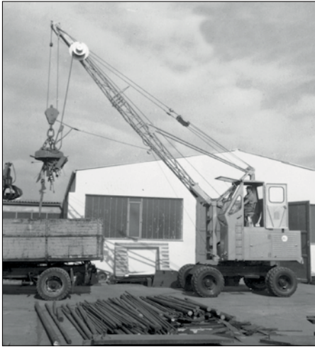
1962: rope-driven S833 with elevated operator cab
