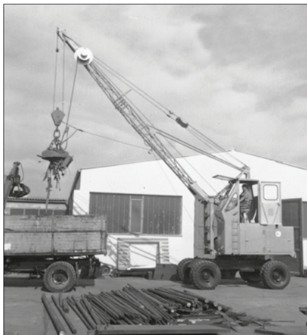
1962: rope-driven S833 with elevated operator cab
